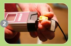
Plug the probe into the handheld console and make sure the battery and probe are working correctly.
