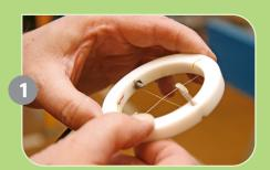
Carefully inspect the Thermoprobe to ensure that the wires are making solid contact with each other. Clean the outer ring and wires with a rag to remove ink or lint.
