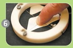
Push the probe wires into the wet ink film. Make sure the wires are embedded in the ink.
