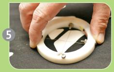
Position the probe over the area with the most ink density.
