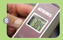
Carefully monitor the display as the print moves down the dryer tunnel. Make sure the peak temperature meets or exceeds the recommended cure temperature for the ink(s) being used.
