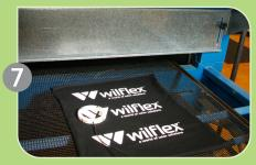
Validate the cure temperature by running a test print through the dryer using the same belt speed as the production run.
