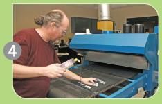
Prepare a test print to simulate the actual production run. Be sure to use the same fabric and printing sequence as the production run.
